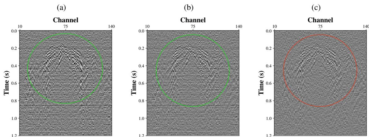
Figure 3: Weak event in the DAS data. a) Event identified with *normal* processing, b) Event identified with the *fx* processing, c) Event not identified with *mix* processing
