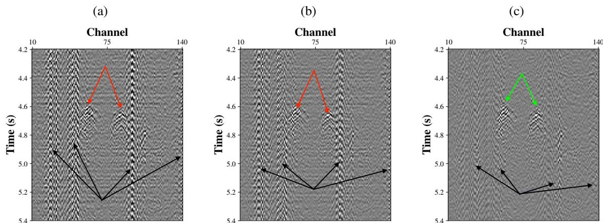
Figure 2: DAS Event only identified by *mix* trained data & model. a) Event with *normal* processing, black arrow points to channel band noise, red arrow points to undetected event. b) Event with *fx* processing, black arrow points to channel band noise, red arrow points to undetected event. c) Event with *mix* processing, black arrow points to filtered channel band noise, green arrow points to identified event.
